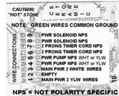
Warning: Discharge static electricity by touching any grounded metal before touching circuitboard or wires
